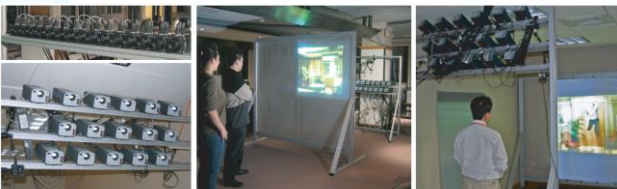
Figure 1: 3D TV system. Left (top to bottom): Array of 16 cameras and projectors. Middle: Rear-projection 3D display with double-lenticular screen. Right: Front-projection 3D display with single-lenticular screen.
